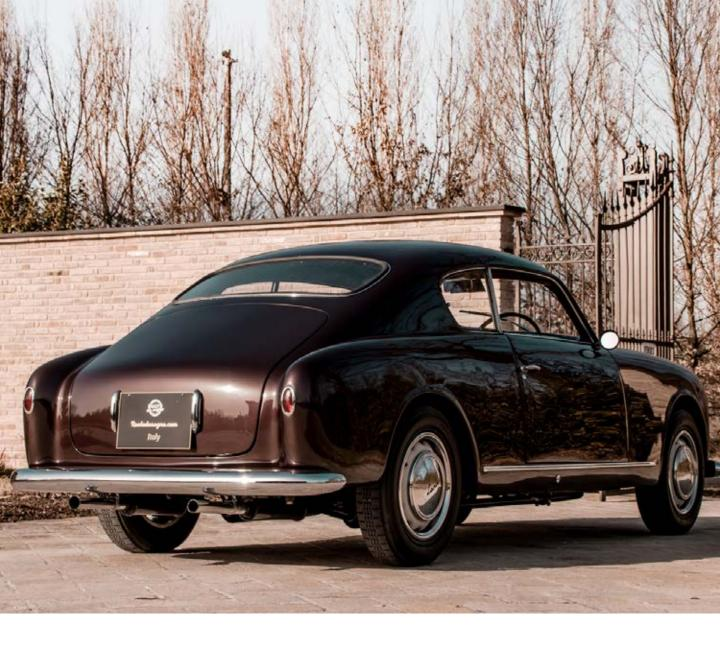
Pininfarina's true masterpiece, which was entrusted with the final contract for the mass production of this model. In March 1952, on the occasion of the Geneva Motor Show, the B20 2nd series was presented. The car has a modified distribution with a slightly increased compression ratio, unchanged driving torque, but a higher power (80 HP instead of 75) that pushes the car up to 162 kph.
