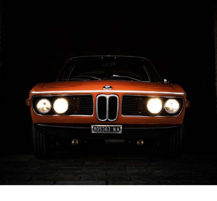
n 1971 the already tested BMW 2800 CS was replaced by the new 3.0 CS and 3.0 CSI models which had a displacement increased to 2986 cm<sup>3</sup>, but, while the first maintained carburetor power and delivered 180 HP, the second fitted an injection mechanics coming to deliver well 200CV.
